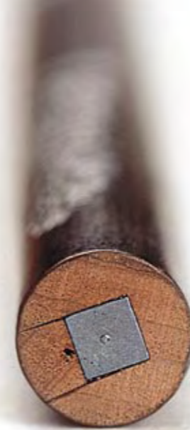
Pencil leads today are usually circular in shape, but square and triangular leads were often used in the past.
