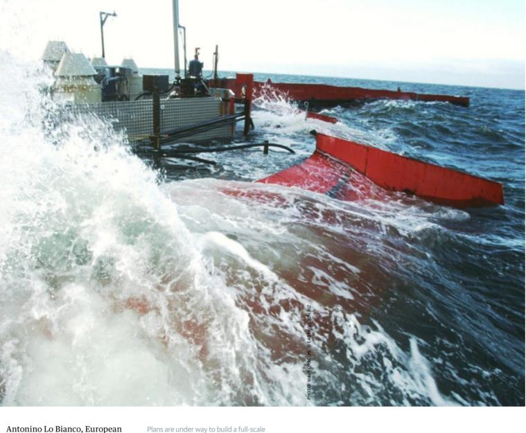
commercial unit of the Wave Dragon off the coast of Wales with a 7-megawatt capacity. The machine contains a turbine which is spun by the crashing waves.
